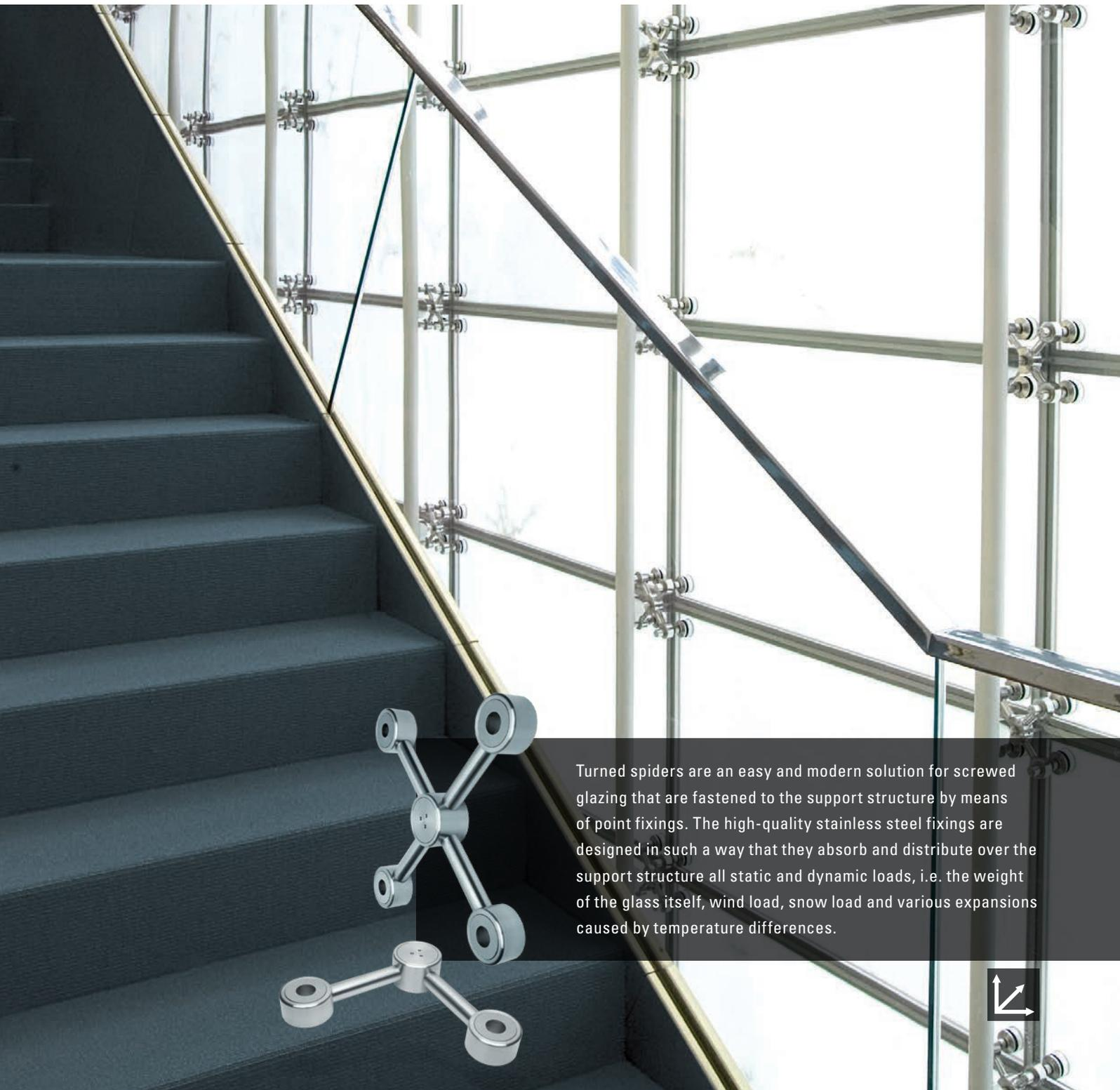
Turned spiders are an easy and modern solution for screwed glazing that are fastened to the support structure by means of point fixings. The high-quality stainless steel fixings are designed in such a way that they absorb and distribute over the support structure all static and dynamic loads, i.e. the weight of the glass itself, wind load, snow load and various expansions caused by temperature differences.
